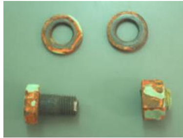
Photo 7-3 Sample bolt with Delayed Fatigue Fracture
