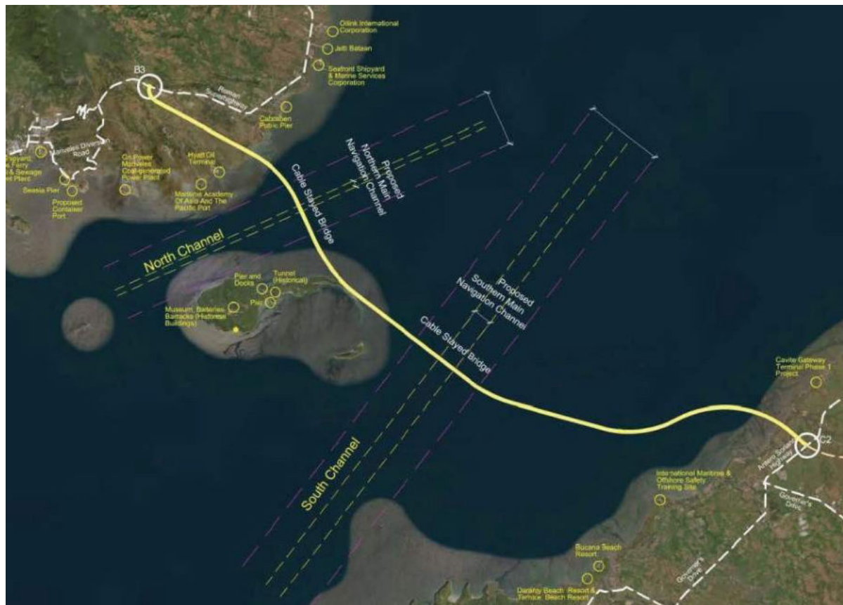
Exhibit 3-3 Plan View of BCIB Showing Navigation Channels
