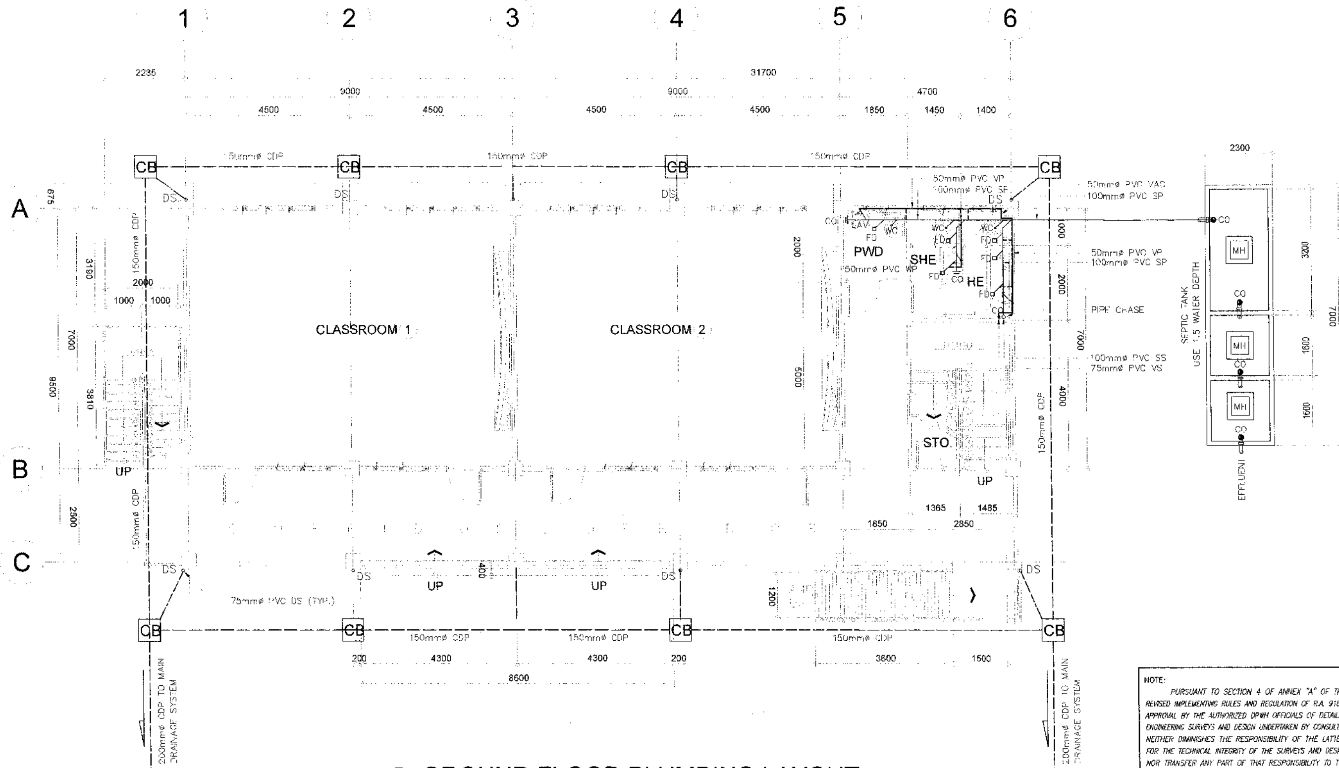
1 P1 GROUND FLOOR PLUMBING LAYOUT SCALE 1:100 METERS
