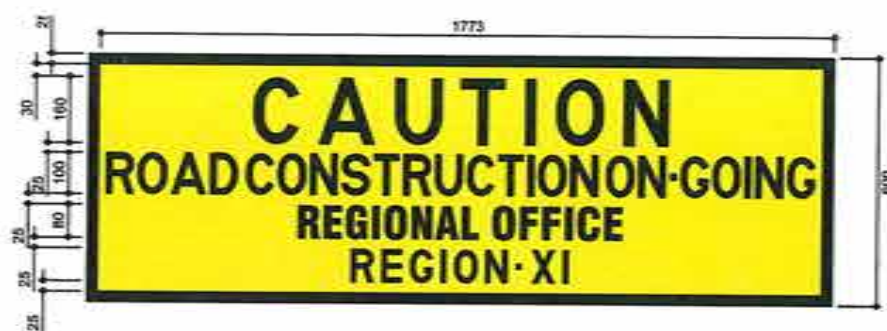
ADVANCE WARNING SIGN
