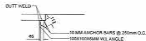
3 BUTT DETAIL SCALE 1:20
