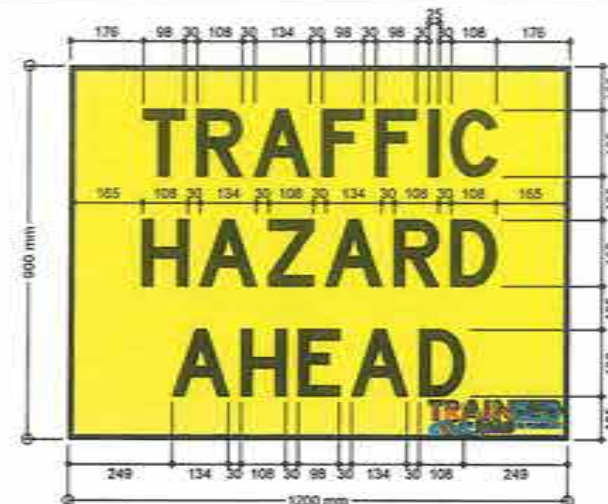
TRAFFIC HAZARD AHEAD (T1-10)
