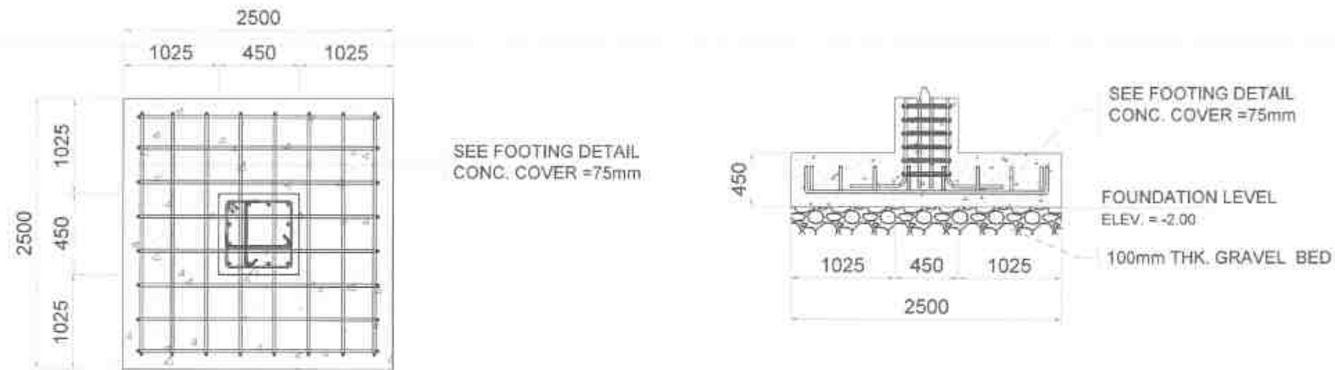
01 0-3 TYPICAL COLUMN FOOTING DETAIL SCALE 1:50 mm
